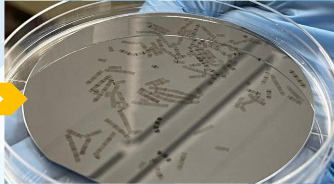
As shown in the photos above, many serial sections can be gathered on a wafer.
