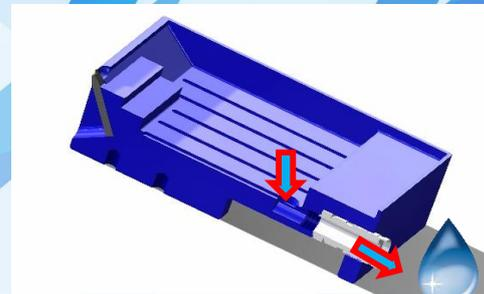
Serial sections can be collected easily, wrinkle-free, and quickly using a drainage mechanism.
