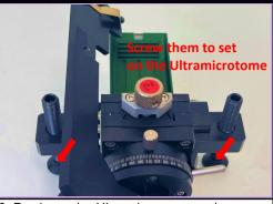
Put it on the Ultramicrotome and turn the screw to stabilize.
