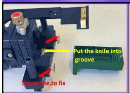
Loosen the screw and set the knife to CUESTA and tighten the screw to fix it.
