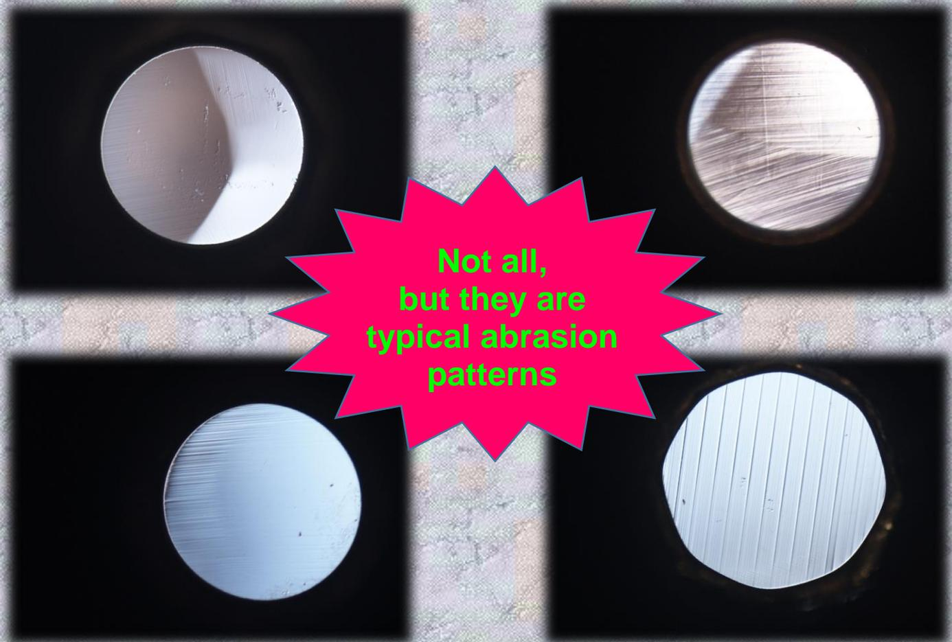
Above photos are condition of original shoe after hundreds hours using. Below picture is Syntek direct acting shoe after 5,000 hours. You see the big difference between above pictures and below one.
