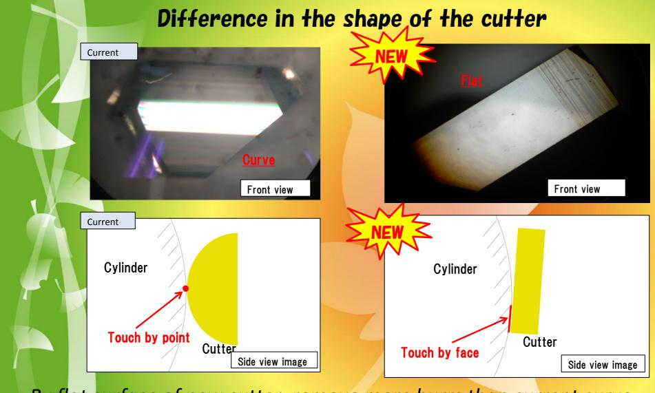
By flat surface of new cutter, remove more burrs than current curve surface efficiently.
