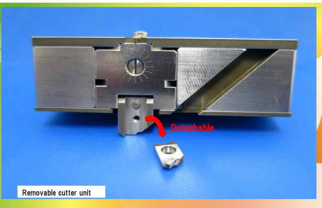
If you want to re-polish the cutter, only remove the cutter unit with a screwdriver.
